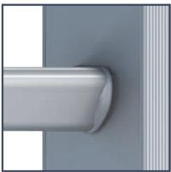
The type of rung folding increases the contact area of the rung on the inner stile face, so that higher forces can be transmitted.
