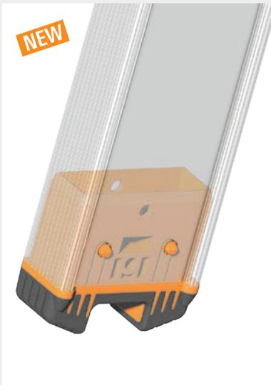
The Layher Combigrip ladder foot is made of a 2-component plastic: a hard inner section (orange) for secure mounting inside the stile, and a soft outer covering (black), non-slip on every floor surface.
