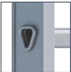
The special design of the ladder stile section permits heavy loading with a low ladder weight. Beading along the outer stile face prevents damage to the rung flanges, for example when they are slid over the edges of the truck loading area.
