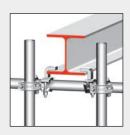
The **clamp couplers 3** for 48.3 mm scaffolding tubes are particularly advantageous for large flange widths. The connection to the flange is always made using two clamping couplers. Permissible load 9 kN per clamping coupler
