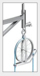
Bracket 12 with hoist wheel 13 for manual vertical transport of scaffolding material weighing up to 50 kg. Loads additionally applied to the scaffolding must be transmitted into the structure or into the ground by special measures, and additional anchoring may be necessary.
