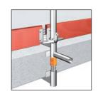
When attached the floors, toe boards must be provided, and the vertical stile must be attached over the spindle.
