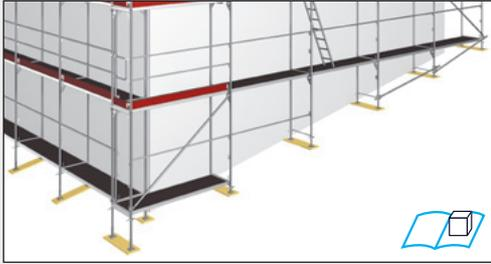
The scaffolding can be adapted to the lie of the land with 0.66 m, 1.00 m and 1.50 m adjustment frames. Assembly always begins at the highest point. The 1.50 x 1.09 m assembly frame has two guardrail wedge housings, making it suitable for use in bricklayer's scaffolding.
