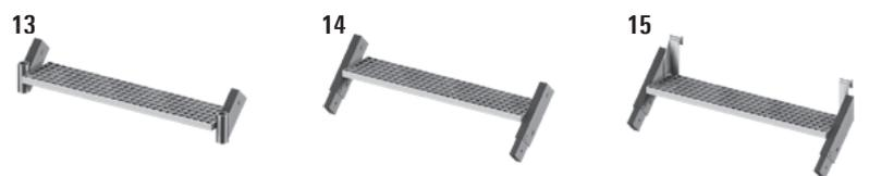
Height differences from 0.60 m to 1.60 m can be bridged. Load-bearing capacity: 3.0 kN/m<sup>2</sup>. Design: steel, hot-dip galvanized. Connection of elements with bolt, dia. 12 x 55 mm and safety clip 2.8 mm (2 per joint). They are already included in the scope of delivery.
